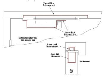
Note: Failure to install intumescent protection identified above will invalidate this certificate
