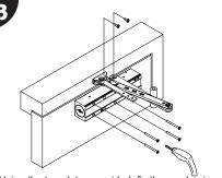
Using the templates provided, fix the mechanism to the door as well as the armset and any necessary brackets.
