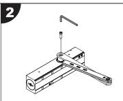
Arm is fitted in pinion with hex head screws.
