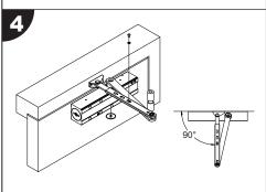
Attach the armset to the mechanism ensuring the pre-loading requirement has been completed.
