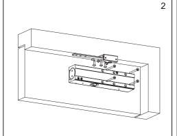
Using the templates provided, fix the mechanism to the door as well as the armset and parallel arm bracket.
