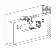
Using the templates provided, fix the mechanism to the door as well as the armset and the parallel arm bracket.
