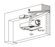
Rotate the bottom pinion at approximately 90° with a wrench as illustrated and then assemble the main arm
