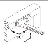
Attach the armset to the mechanism ensuring the pre-loading requirement has been completed.
