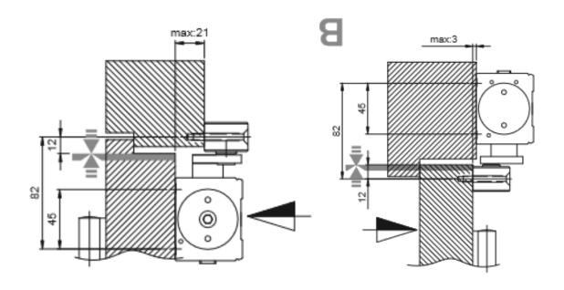
S3406.AB Angle Bracket to suit Deep Head Reveal Section on both 3400 and 3500 Closers
