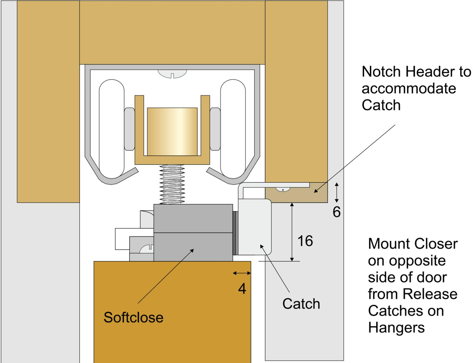
Minimum door size possible is 686mm. If door is between 686mm - 734mm then lose the 25mm spaces between hanger plates and softclose unit and reduce catch distance from jamb to 294mm
