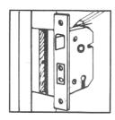
2. Insert lock and mark position of front plate recess.
