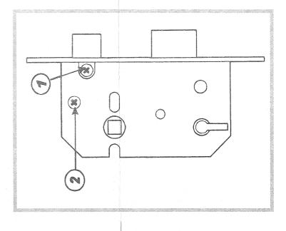
Insert screw into hole (2) and secure.
