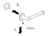
Loosen the set screw on the accessory and remove the backing plate. Position the accessory against the wall and mark outline with pencil.
