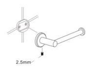
Slide the accessory onto the backing plate and tighten the set screw using Allen Key provided.
