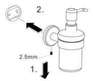
1. Loosen the set screw on the accessory and remove the backing plate. Position the accessory against the wall and mark outline with pencil.
