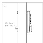
Insert the spindle. Cut to length if it protrudes more than the dimension shown.
