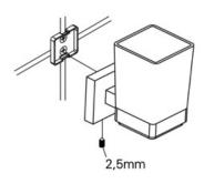
Slide the accessory onto the backing plate and tighten the set screw using Allen Key provided.
