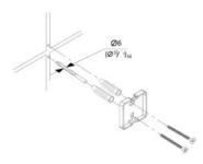
3. Mount to drywall Predrill holes on the wall to fit wall anchors. (15/64" Drill bit recommened). Insert wall anchors into the wall.
