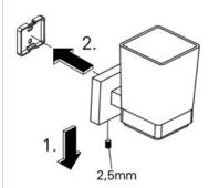
1. Loosen the set screw on the accessory and remove the backing plate. Position the accessory against the wall and mark outline with pencil.
