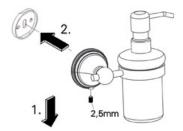
Loosen the set screw on the accessory and remove the backing plate. Position the accessory against the wall and mark outline with pencil.
